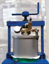
LMPF, pressure filter 4 - liter table model
